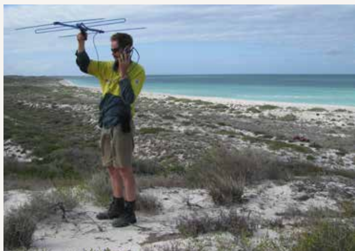
Above Michael Johnston using an antenna and a receiver to locate radio-collared animals.
